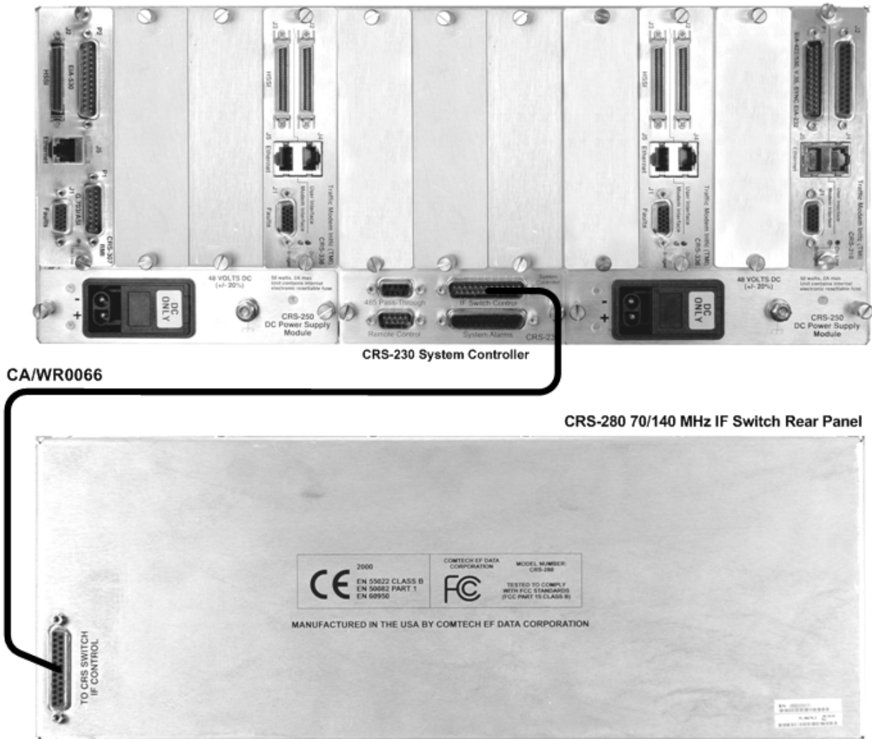
Figure 4-1. Control Cable Connection Example for CRS-300 to CRS-280
